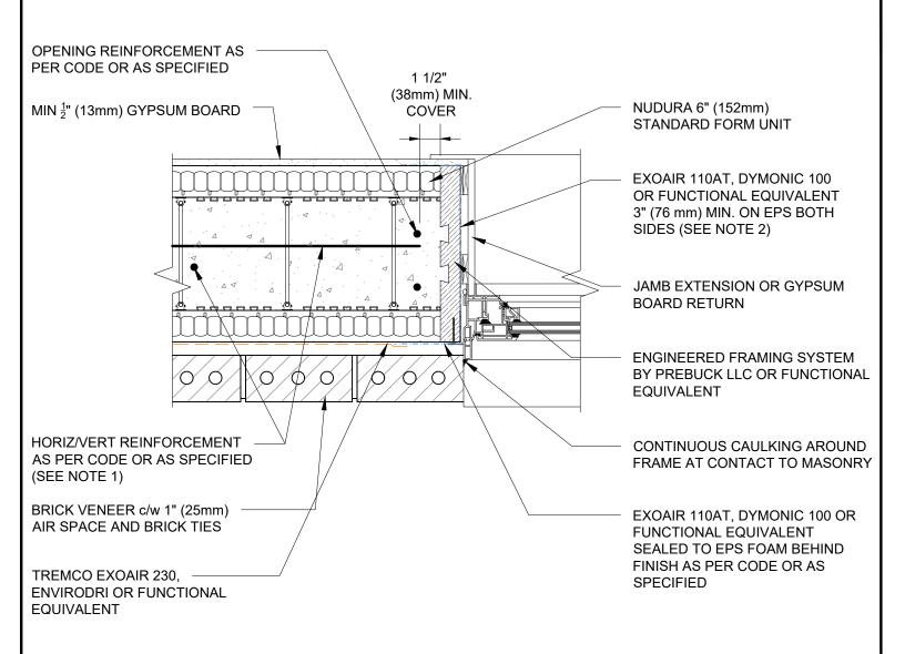
1) FOR OPTIMAL REINFORCEMENT PLACEMENT IN THE NUDURA FORM, SPACING OF HORIZONTAL REINFORCEMENT TO BE SPECIFIED AT 18" (457mm) O.C. AND VERTICAL REINFORCEMENT TO BE SPECIFIED AT MULTIPLES OF 8" (203mm) O.C. REFER TO NUDURA REINFORCEMENT PLACEMENT DETAILS.
