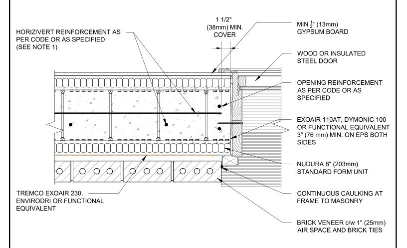
1) FOR OPTIMAL REINFORCEMENT PLACEMENT IN THE NUDURA FORM, SPACING OF HORIZONTAL REINFORCEMENT TO BE SPECIFIED AT 18" (457mm) O.C. AND VERTICAL REINFORCEMENT TO BE SPECIFIED AT MULTIPLES OF 8" (203mm) O.C. REFER TO NUDURA REINFORCEMENT PLACEMENT DETAILS.
