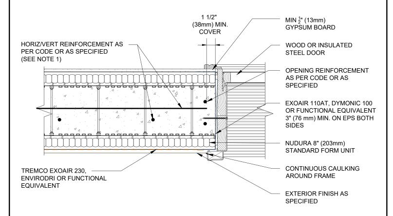
1) FOR OPTIMAL REINFORCEMENT PLACEMENT IN THE NUDURA FORM, SPACING OF HORIZONTAL REINFORCEMENT TO BE SPECIFIED AT 18" (457mm) O.C. AND VERTICAL REINFORCEMENT TO BE SPECIFIED AT MULTIPLES OF 8" (203mm) O.C. REFER TO NUDURA REINFORCEMENT PLACEMENT DETAILS.
